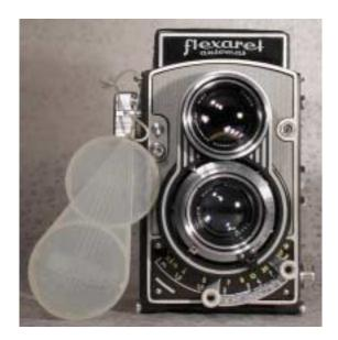
The Flexaret twin lens reflex cameras are a product of the Czechoslovakian company Meopta (manufacturers of enlarging equipment). The Flexaret Automat VI was in production from 1961-1967. This camera is a multiformat camera, 6x6 and 35 mm.
